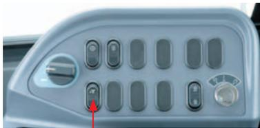
Dual mode engine power selection switch
